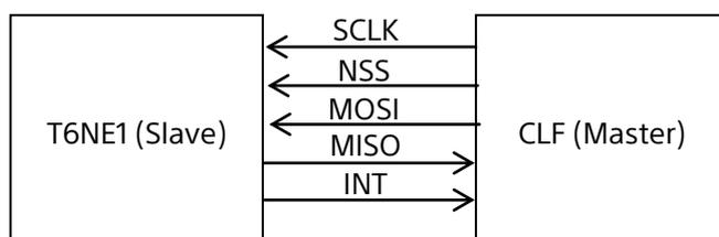
**Figure 3 : Connection Description between T6NE1 and CLF**
