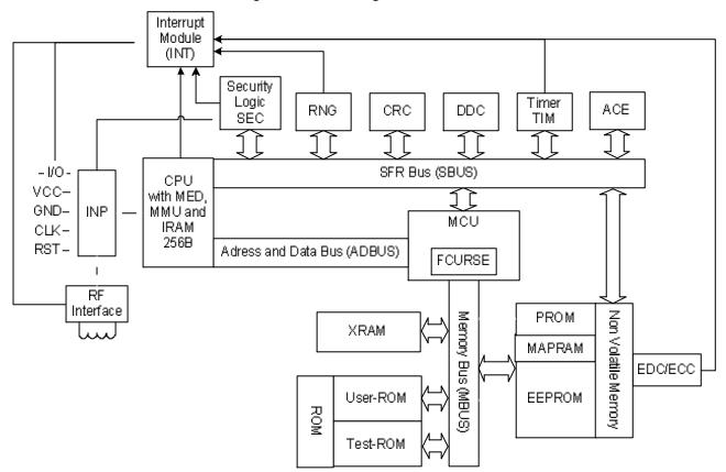
Figure 1: Block diagram of the TOE
