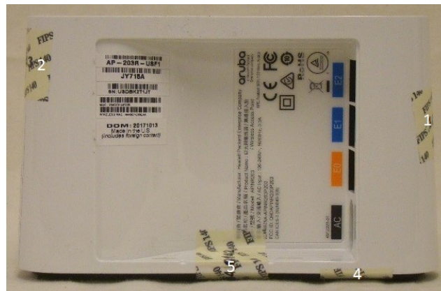
Figure 11 – Back View of AP-203R with TELs
