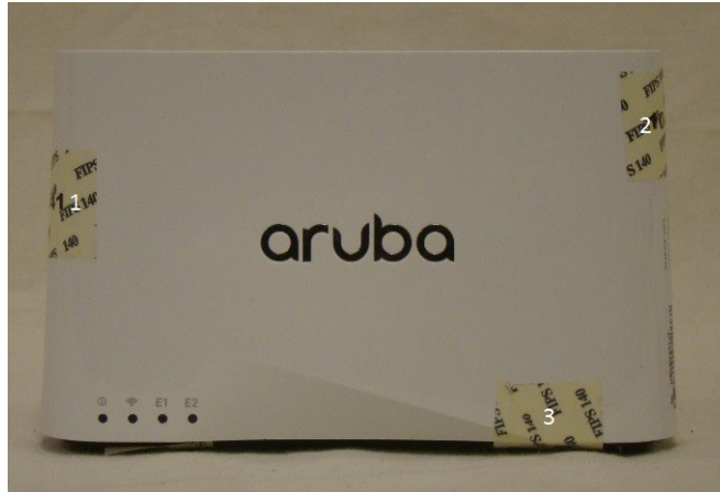
Figure 10 – Front View of AP-203R with TELs
