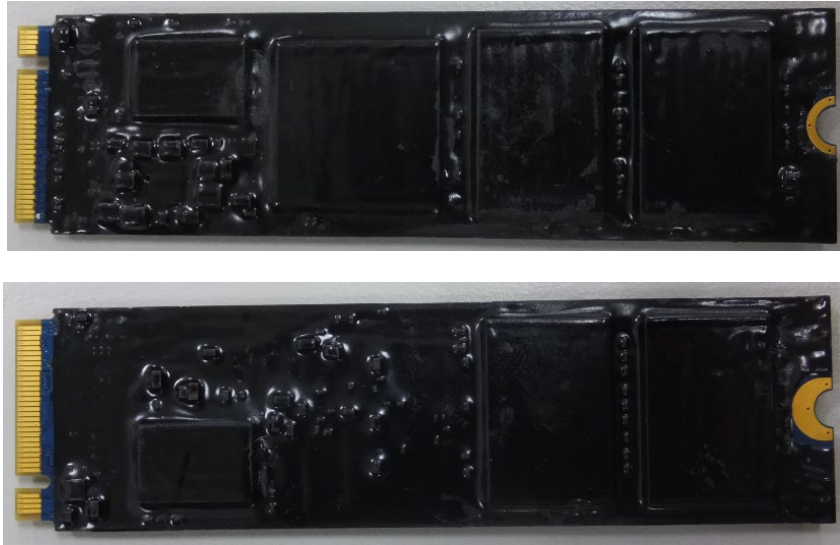
Exhibit 4 - Specification of the KSED300-N M.2 2280 NVMe NAND FLASH SSD Series Cryptographic Boundary (From top to bottom: top side, bottom side).
