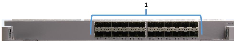
Figure 3-3: S7703 / S7706 / S7712 LPU Card Ports
