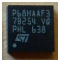
Figure 10: Picture of the Cryptographic Module (VQFN32) – Marking P68HAAF3
