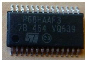
Figure 9: Picture of the Cryptographic Module (TSSOP28) – Marking P68HAAF3
