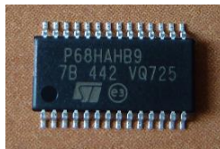
Figure 6: Picture of the Cryptographic Module (VQFN32) – Marking P68HAHB9
