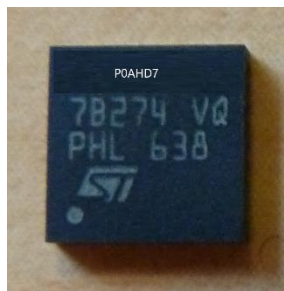
Figure 14: Picture of the Cryptographic Module (VQFN32) – Marking P0AHD7
