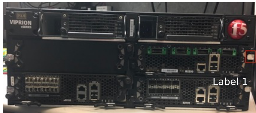
Figure 15 - Tamper labels on BIG-IP 10350v-F. Top: BIG-IP 10350v-F with faceplate from Picture Table 1 removed and the tamper label 1 affixed to secure the housing for externally-accessible storage drives. Middle, Bottom: tamper labels shown at the intersection between cover and chassis (2 opposite sides of the platform -labels 3 and 4- and front -label 2-).
