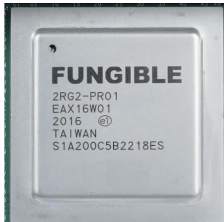
Figure 2 -Fungible S1 Data Processing Unit (Fungible S1 rev A0)
