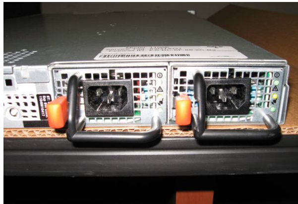
Figure 4 – Rear Panel of McAfee Firewall Enterprise 1100E
