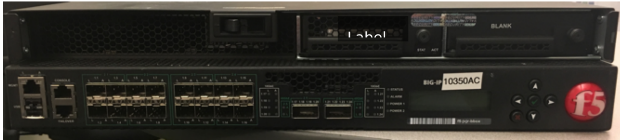
Figure 5 - BIG-IP 10350v-F with faceplate removed (1 of 4 tamper label shown)
