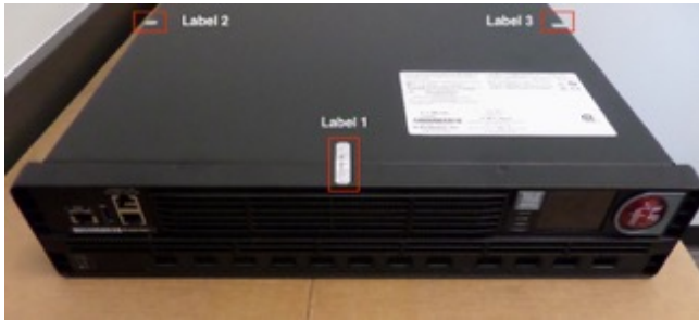
Figure 12-BIG-IP i15800 (Front tamper labels 1-3 labels shown)
