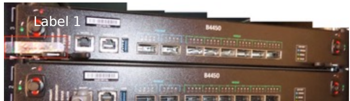
Figure 15-VIPRION B4450 front (1 of 5 tamper labels shown)
