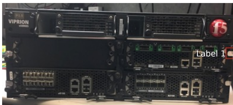
Figure 8-VIPRION B2250 in chassis (1 of 6 tamper labels shown)
