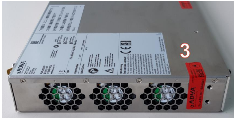
Figure 24: Placement seals, shelf 1 HU, placement 3
