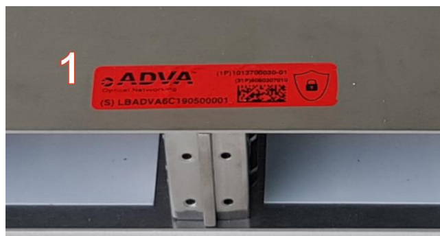
Figure 22: Placement seals, shelf 1 HU, placement 1
