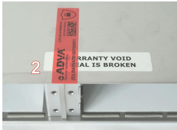
Figure 30: Placement of seal SH1HU-R/PF right side position
