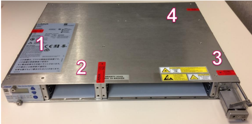
Figure 26: Placement of seals SH1HU-R/PF front-top view
