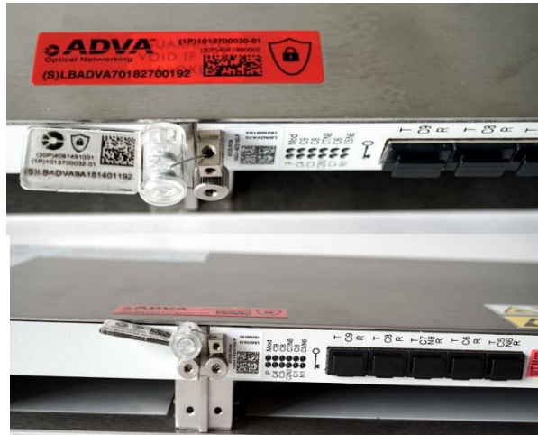
Figure 35: Placement of twist seal in SH1HU configuration
