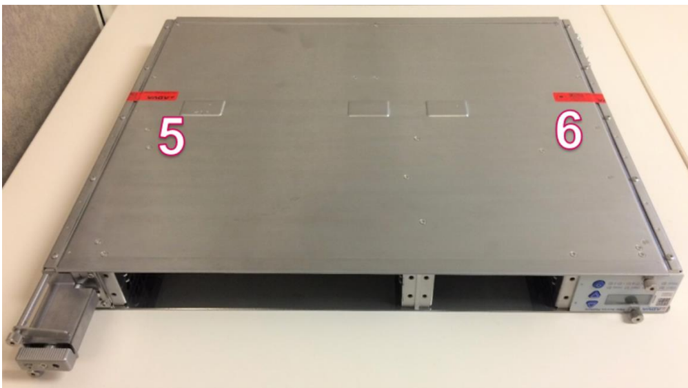
Figure 27: Placement of seals SH1HU-R/PF front-bottom
