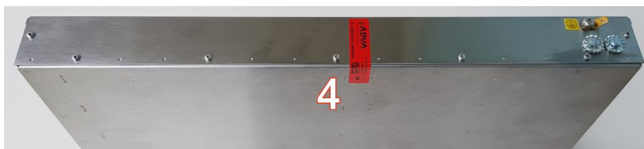
Figure 25: Placement seals, shelf 1 HU, placement 4
