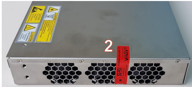
Figure 23: Placement seals, shelf 1 HU, placement 2
