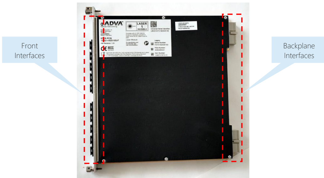
Figure 8: 9TCE top view with marked interfaces
