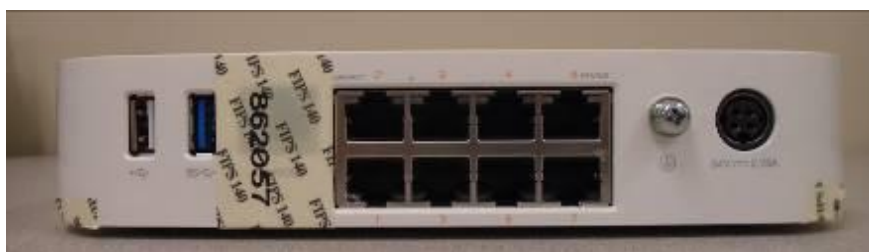
Figure 13 - Required TELs for the Aruba 7008 Mobility Controller – Front
