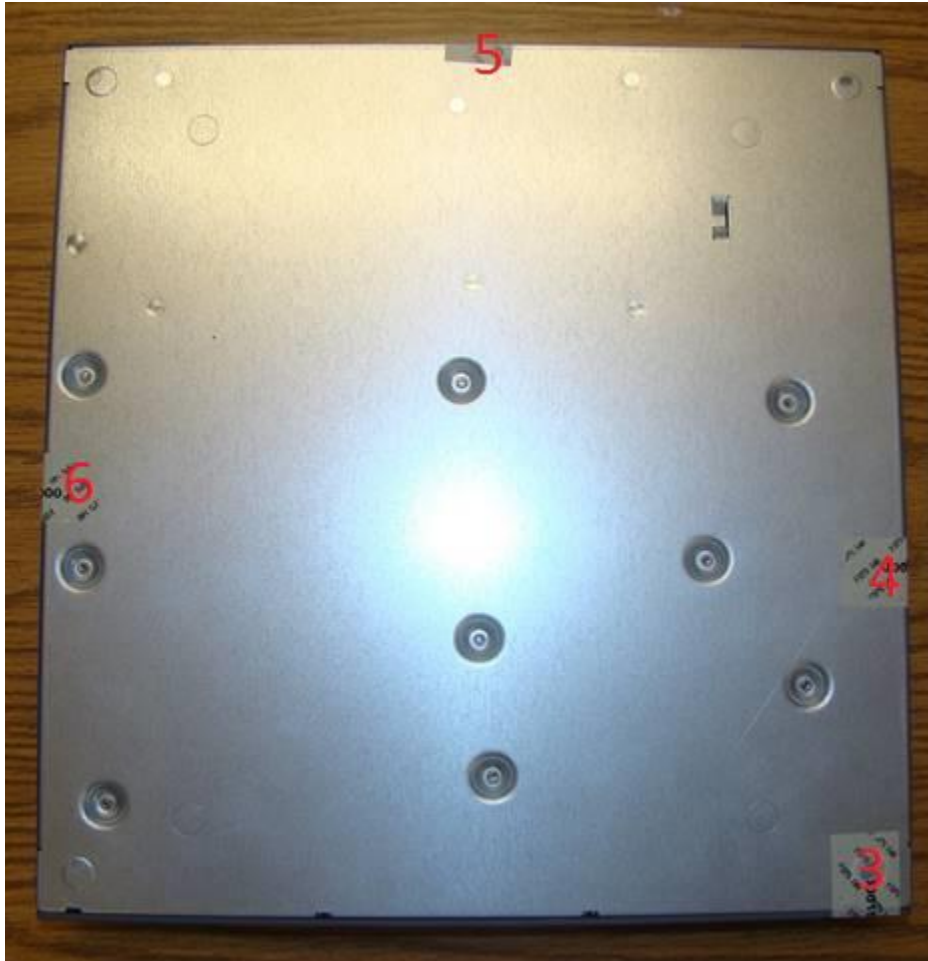
Figure 16 - Required TELs for the Aruba 7010 Mobility Controller – Bottom
