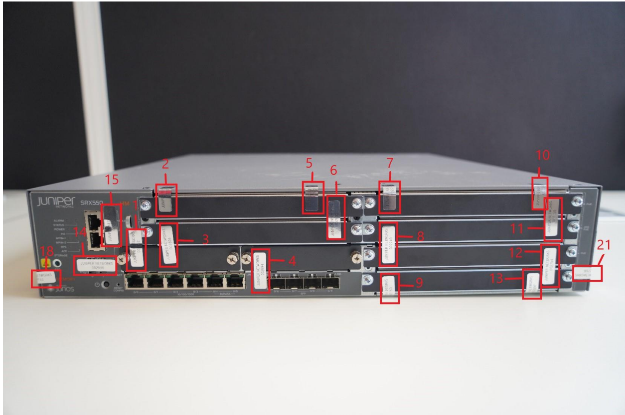
Figure 26 – SRX550M Tamper-Evident Seal Placement (Front, Fifteen (15) Seals: TEL 1-15)
