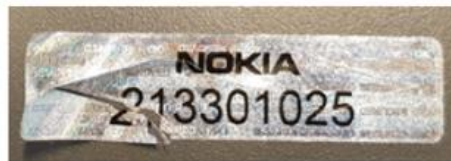
Figure 13: Tamper-evident label: broken (close-up view)
