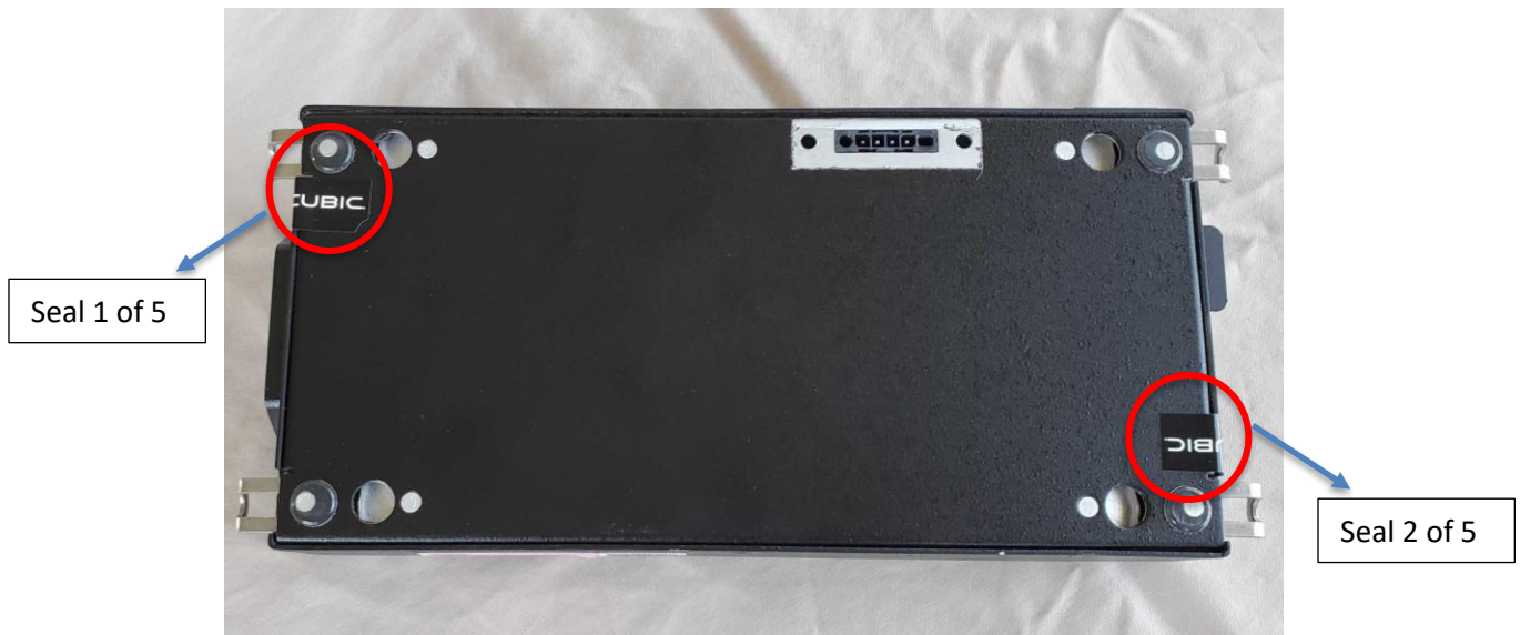
Figure 9 – M3-SE-MFGW Factory-Applied Tamper-Evident Seals – Bottom Straight View
