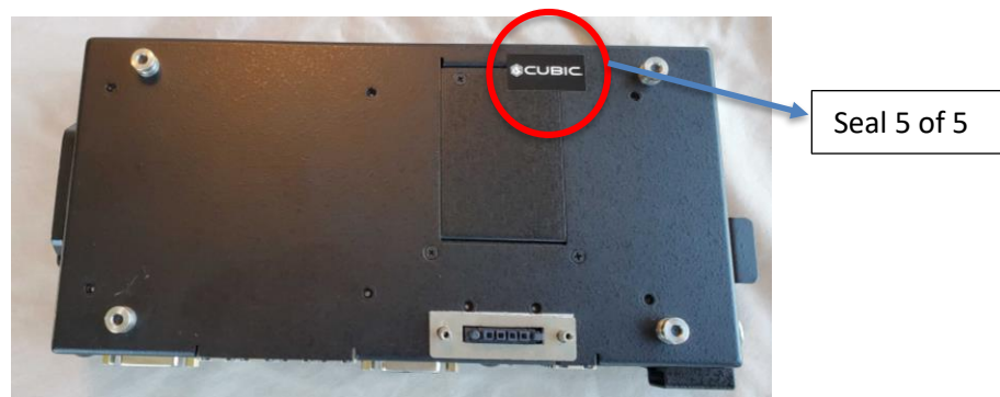
Figure 13 – M3-SE-MFGW Factory Applied Tamper-Evident Seal – Radio Access Cover
