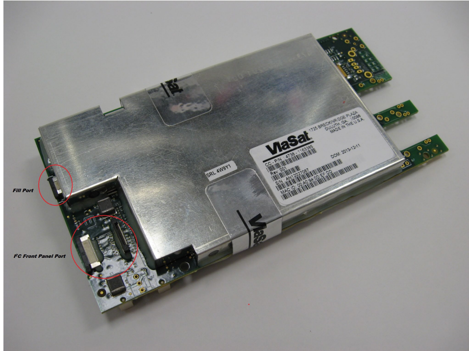
Figure 1-3 Top Side of the 1163385 Cryptographic Module
