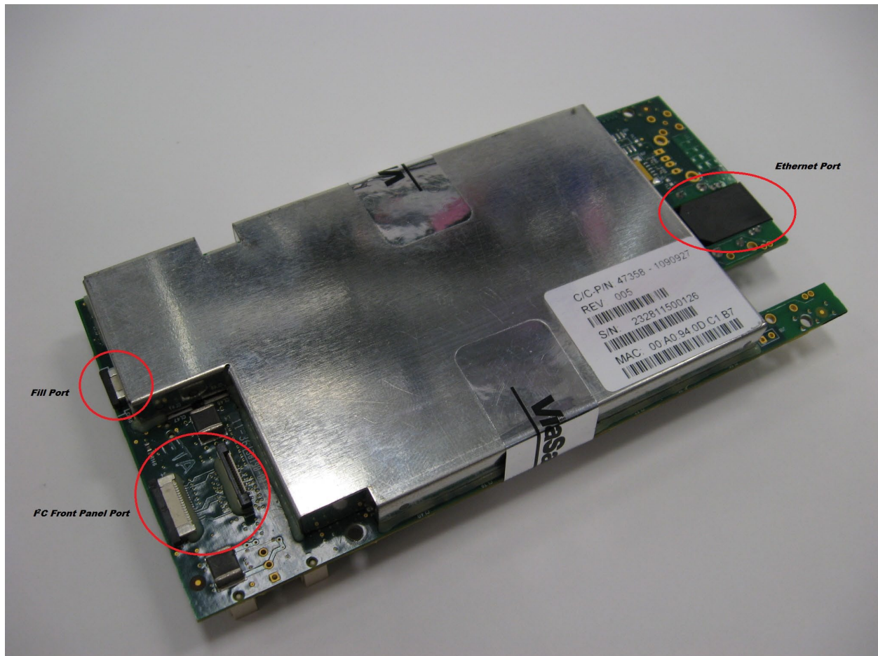
Figure 1-1 Top Side of the 1090927 Cryptographic Module
