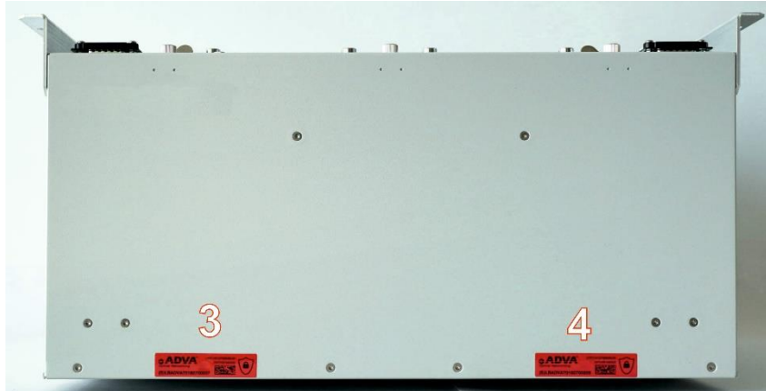
Figure 28: Seals cover rear edge shelf 9 HU
