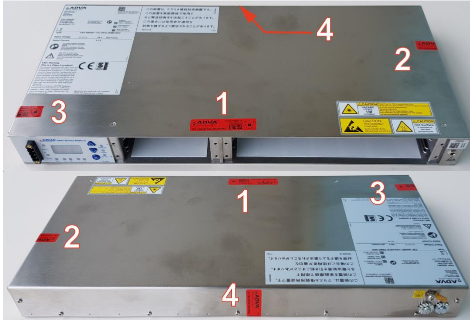
Figure 17: Placement of seals on shelf 1 HU, top views
