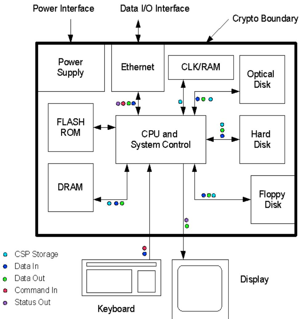
Figure 2: Software Block Diagram
