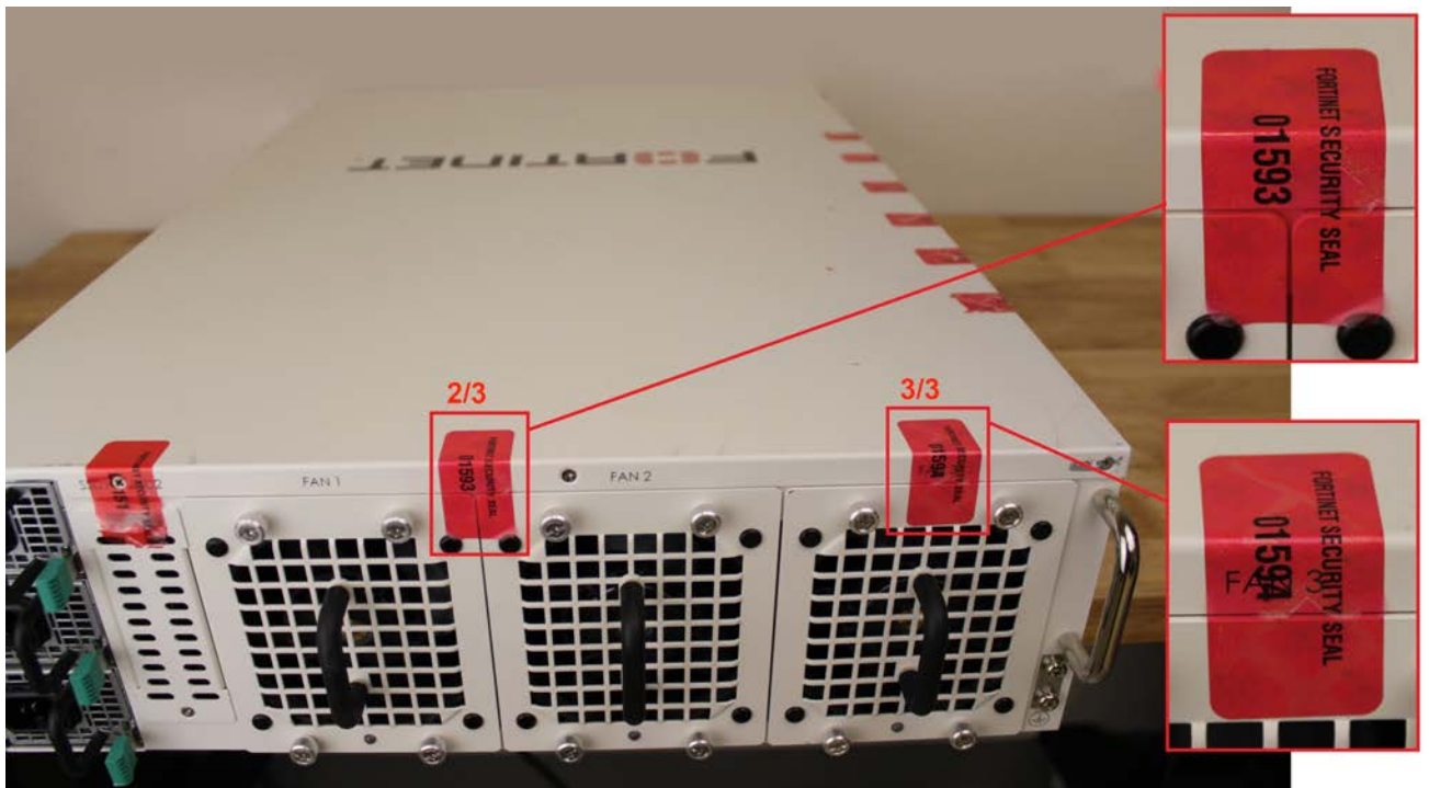
Figure 3 - FortiGate-6300F/6301F/6500F/6501F external enclosure seal 2 and 3, top, rear
