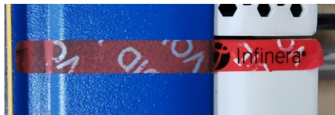
Figure 6 – Tamper-evident label: broken (close-up view)
